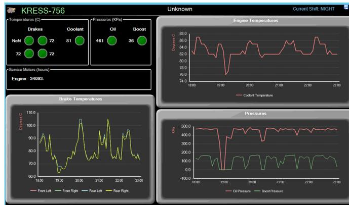
Figure 1: Haul Truck Maintenance Parameters
