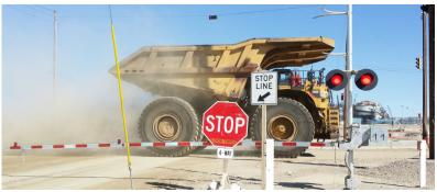
This allowed 3D-P to develop an on-board application which determined if a haul truck was heading towards the intersection based on the Endpoint's location awareness. Upon approach, the Intelligent Endpoint messages the traffic light controller. Construction
