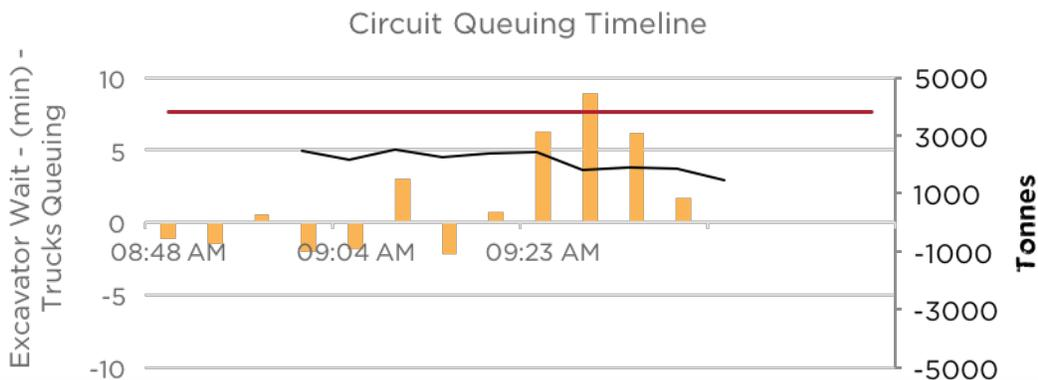
Fig. 3 - The study revealed significant trucks queuing time and moderate excavator waiting periods, highlighting opportunities for improvement.
