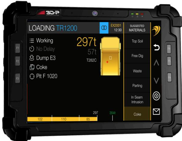
Fig. 2 - The in-cab excavator operator screen provides tonnage and CoG of the truck it's loading in real time.
