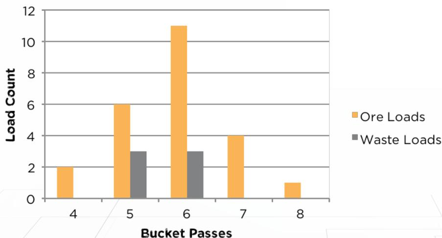
Fig. 1 - Despite a waste target of 6 passes and an ore target of 5 passes, the excavator proved to be repetitively over its ore target.
