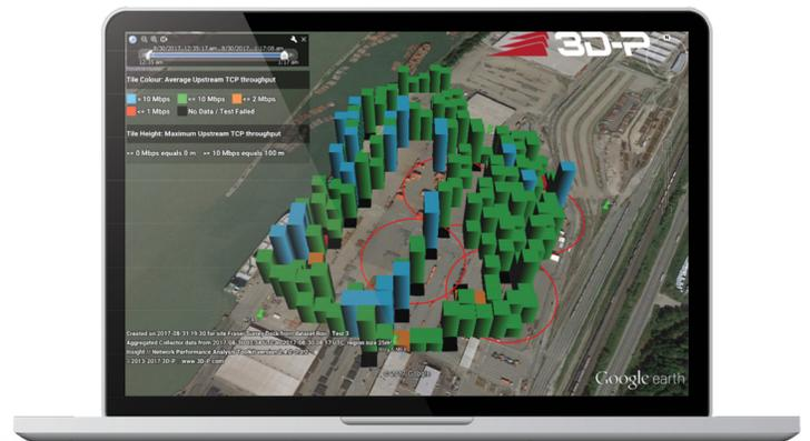
Fig. 1 - Results showed 100% coverage on both channels and throughput averaging between 2 and 20Mbps over the entire site
